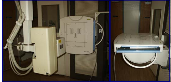
The Thormat Chest Unit, at Hamilton General, is also a room that was retrofitted to Canon DR. This retrofit allowed the Thormat to utilize all of its original features with the added versatility of performing general procedures due to the Rotating/Tilting Bucky (Pictured Right)
